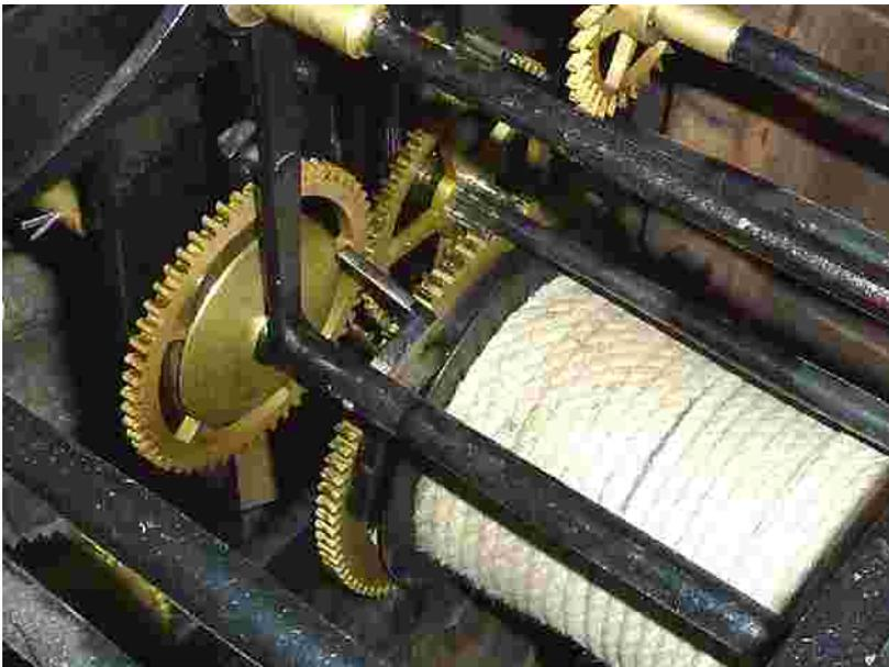
Figure 8 - brass wheels and the rope wound around the barrel.
